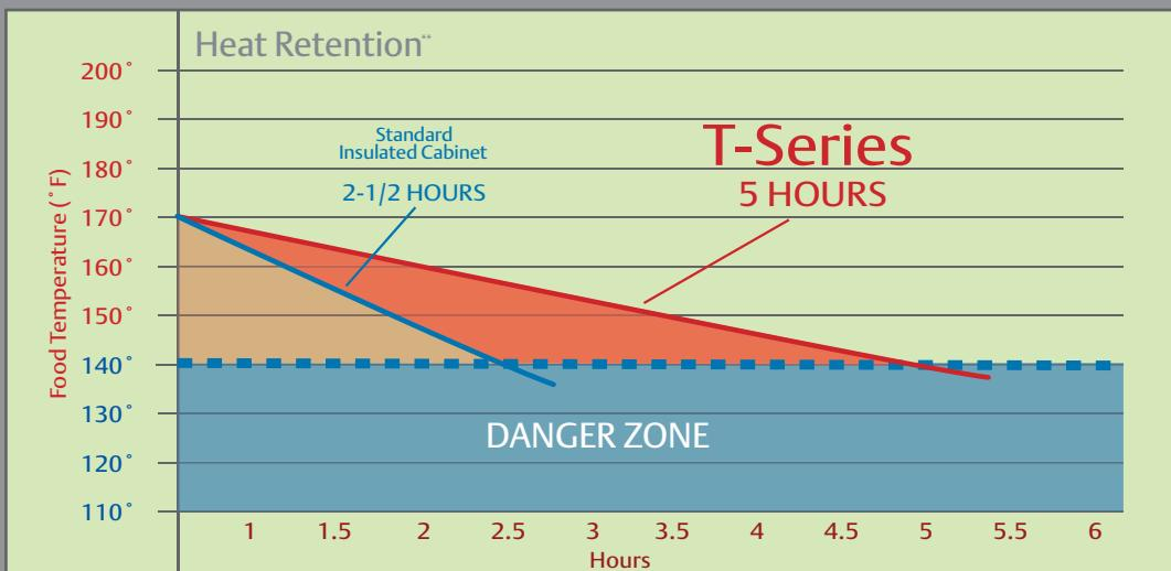
\*\* Average food temperature 170° F, cabinets preheated to 180° F. Four 12" x 20" x 4" uncovered steam pans were placed inside cabinets. Additional food mass and covered pans may result in longer heat retention.
