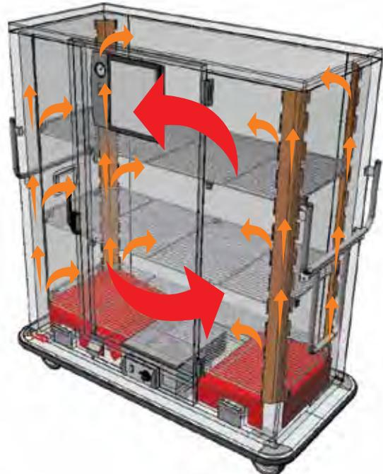
canned fuel back-up system available, offering superior heat stratification and control. Quad-Heat™ corner chimneys utilize the “dead space” in the corners of the cabinet, surrounding plated meals with even heat distribution, minimizing the size of the cabinet, and maximizing heat efficiency. Our canned fuel drawers can be accessed without opening the cabinet doors for monitoring.
