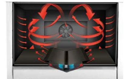
High performance "I" shaped burner provides even heat throughout the 35,000 BTU oven.
