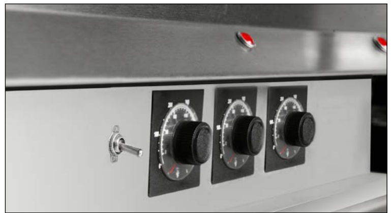
Solid state temperature control & electronic spark igniter for each 12" of griddle width.
